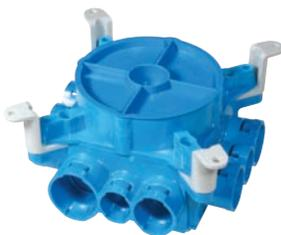
Carlton Mud Box Assemblies w/ Mounting Feet are specifically engineered and designed for use in Tunnel Form applications. The mounting feet are located on all four corners and allow the box to attach directly to the wall of the form using pop rivets. The pop rivets help keep the box in position during the pour and provide a safe, secure, and rust resistant mount.
