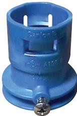
**Carlson ENT to EMT Transition Adapters** are designed to easily transition from Carlson Flex-Plus® Blue ENT to EMT using Carlson's "Quick Connect" snap-in design. The EMT is held securely in place using the small screw provided. This helps prevent the EMT from slipping/shifting out of the adapter. All ENT to EMT adapters are manufactured out of polycarbonate material to provide extra strength and durability. They're concrete tight, and available in sizes 1/2", 3/4" and 1".
