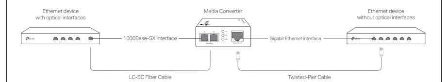
Note: MC220L needs to be plugged in with an SFP module to work normally. It is recommended to use a TP-Link SFP module on MC220L, because other vendors' SFP modules may be incompatible.
