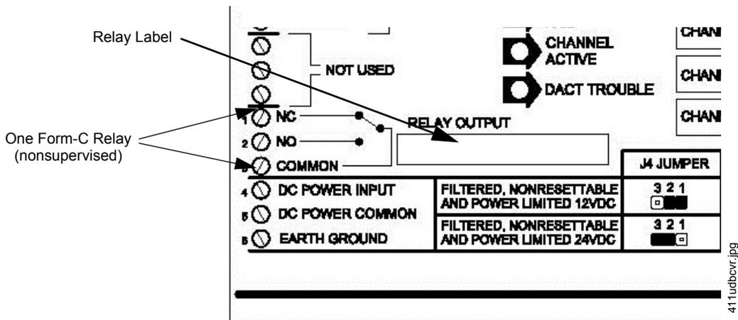
Figure 2.3 Programmable Relay
