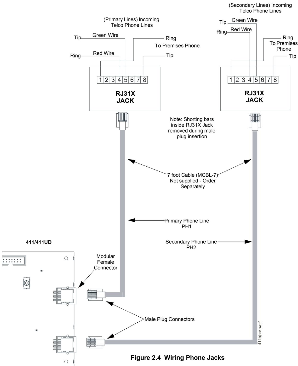
Figure 2.4 Wiring Phone Jacks
