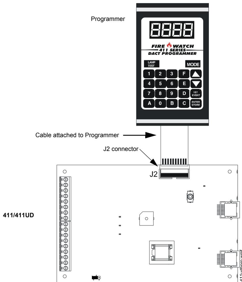
**Figure 2.5 Programmer Connection to 411/411UD**
