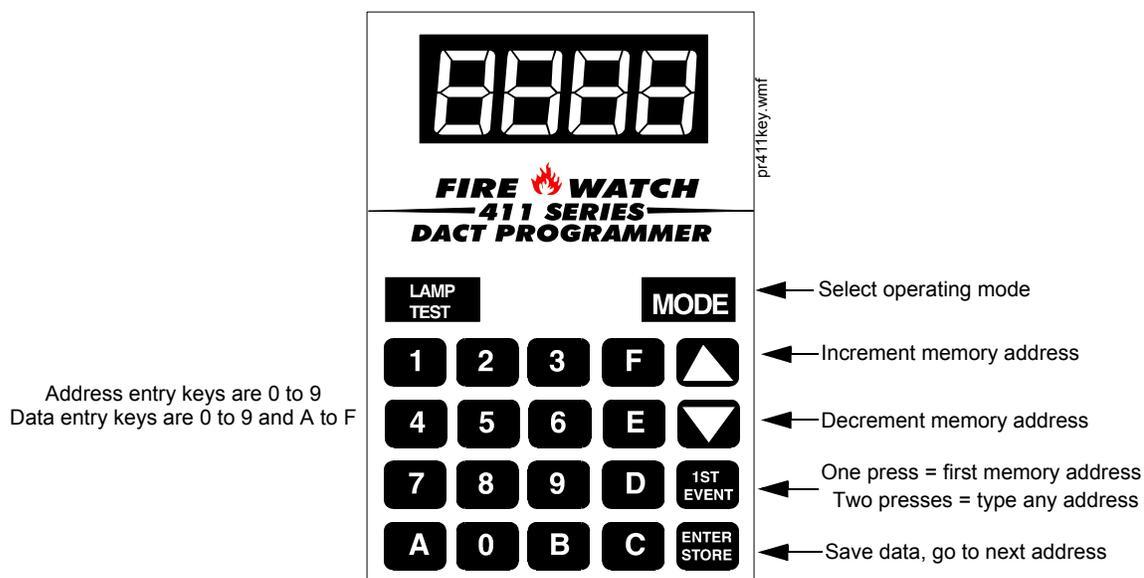
Figure 3.1 Programmer Keypad
