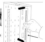
7. Install camlock onto box lid and mount any remaining devices.
