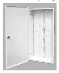
8. If desired, two (2) #10 sheet metal screws can be installed in the right side of the lid (upper and lower) to make the box more secure against tamper. In addition, the SWB28 provides mounting holes for two tamper switches.
