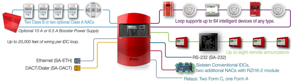
Each VS1 panel ships with one device loop controller that supports 64 devices of any type. This panel's device capacity cannot be expanded.
