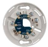
This base includes a relay. Normally-open or closed operation is selected during installation. The dry contact is rated for 1 amp (pilot duty) @ 30 Vdc. The relay's position is supervised to avoid accidentally jarring it out of position. The relay base does not support the SIGA-LED remote LED. It mounts to North American one-gang boxes, 3½ or 4-inch octagon boxes, or 4-inch square electrical boxes. Bases for 4-inch square boxes include a trim skirt.
