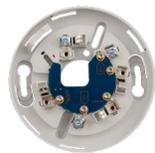
Isolator detector bases provide room-side wiring terminals and includes a built-in line fault isolator. Models with integral switches allow the detector to be removed from its base without causing the isolator to operate. Mounts to North American one-gang box, 3½ or 4-inch octagon boxes, or 4-inch square electrical boxes.
