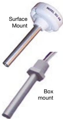
Series 302 heat detectors are designed for use in normal environments as well as environments where the detectors are subject to weather, moisture (internal condensation), and explosive atmospheres. They are normally-open devices designed to close an electrical circuit upon activation. All models feature rate compensation and are available with either 135 °F (57.2 °C) or 194 °F (90 °C) ratings. They are self restoring, hermetically sealed, shock and corrosion resistant, and are tamperproof.
