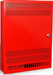
The Remote Booster Power Supply is a self-contained 24 Vdc power supply designed to augment fire alarm audible and visual power requirements as well as provide power for auxiliary, access control and security applications. The booster contains all of the necessary circuits to monitor and charge batteries, control and supervise four Class B or two Class A NAC circuits and monitor two controlling inputs from external sources.
