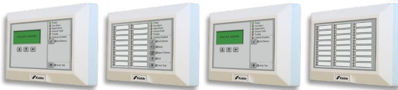
There are three R-Series annunciator models, plus an LED-based expander. Up to two expanders can be connected to any annunciator. The expander includes 24 pairs of LEDs that extend the capabilities of any of the annunciators.
