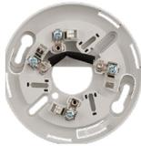
Standard detector bases provide roomside wiring terminals. They mount to North American one-gang box, 3½ or 4-inch octagon boxes, or 4-inch square electric box. Bases for 4-inch square boxes include a trim skirt to conceal the electric box and provide a finished appearance.
