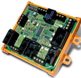
The GSA-REL Releasing Module is an Intelligent addressable device that works with fire suppression systems designed to release extinguishing gas such as Halon. Its primary function is the control of sprinkler pre-action routines and the initiation of suppression system deluge functions. The module is easily configured in the field and offers a wide range of options that
