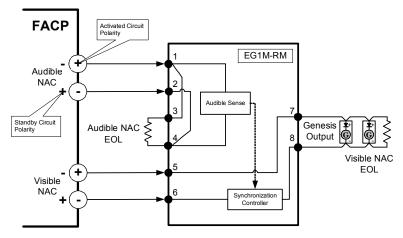
**NOTE:** All Genesis NAC circuit power is derived from the visible NAC connected to terminals 5 and 6. The Genesis NAC current capacity is 2A for the EG1M and 3A for the EG1M-RM. The Audible NAC input terminals (1/2) are used for horn control only and do not draw any significant current.
