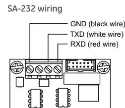
The RS-232 card is installed on the plastic assembly and connects to the main circuit board via a ribbon cable.
