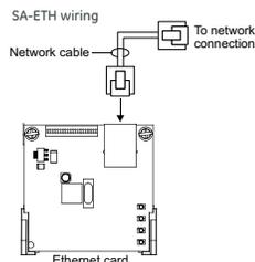
The SA-ETH card provides a standard 10/100 Base T Ethernet network connection for connecting to an intranet, a local network, or the Internet. The card supports IP connectivity for monitoring services by a supervising station to meet NFPA 72 Chapter 26. The Ethernet card uses the FIBRO protocol to communicate with Sur-Gard System receivers (see below). The card can be used to download configuration programming from the VS-CU to the panel.
