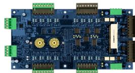
The RZI16-2 Addressable Remote Zone Interface Module is an addressable device that provides connections for sixteen Class B Initiating Device Circuits and two Class B Supervised Output Circuits. The inputs and outputs can be configured individually for several device types.
