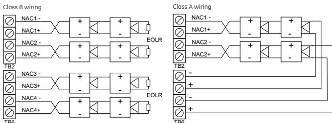
Marking indicates output signal polarity when the circuit is active. Polarity reverses when the circuit is not active. Wire notification appliances accordingly. Notification appliance polarity shown in active state.
