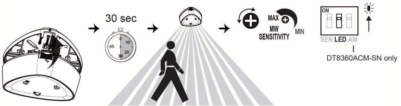
1. Close the sensor and apply power to the sensor. Initialization is complete when the LED stops flashing slowly (about 30 seconds).
