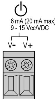
For new polling loop installations, always use shielded twisted pair wiring. In many cases, existing non-twisted pair wiring may be used, but it is more susceptible to interference from other sources, and may be problematic in installations with long wire runs or in high noise environments.
