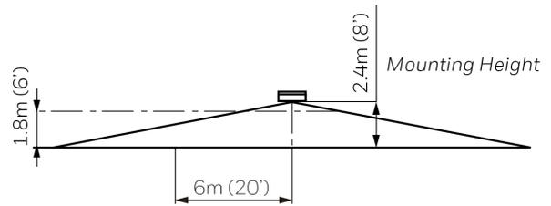
**Note:** Attention detection beams go across access points such as windows, doors during sensor installation.
