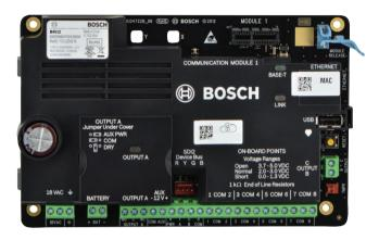
The B4512 Control Panel integrates intrusion and residential fire, providing one simple user interface for both systems. The B4512 provides up to 28 individually identified points that can be split into 2 areas.
