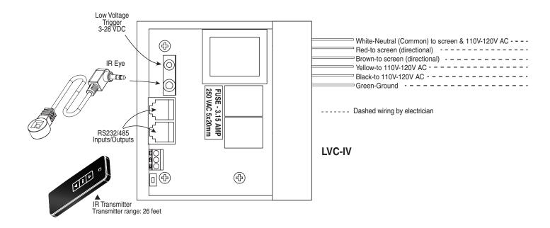
Wire to connect power to LVC-IV should be between 18 AWG and 12 AWG (solid or stranded) 2 conductors with ground. Wire size needs to be sufficient to carry the motor load. Red and Black wires are the "open" and "close" leads from the motor. The LVC-IV comes enclosed in a metal box with appropriate spacing between the wires and any exposed parts of the box. IR Eye is connected to LVC-IV using low voltage modular data or telephone cord (RJ11), which is isolated from the AC power line.
