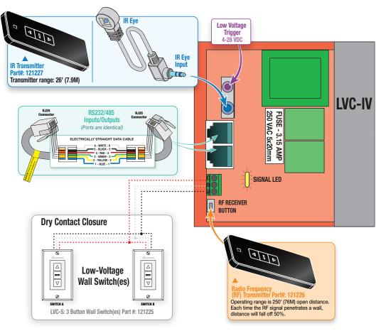
The 230V LVC-IV also used as a Single-Pole, Double-Throw dry closure to control equipment by the same means listed above.
