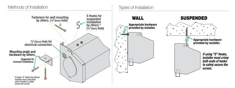
Please Note: If using "S" Hooks, installer must crimp both ends of the "S" hooks to safely secure the screen.
