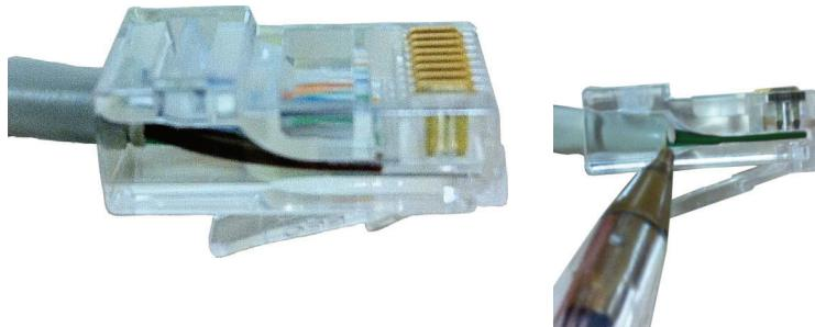
8. Make sure the wires are fully inserted by inspecting the side of the transparent connector. Next, insert the connector into the crimping pliers and, using both hands, crimp the connector so as to secure the wires. The pliers should not open if they did not close fully.
