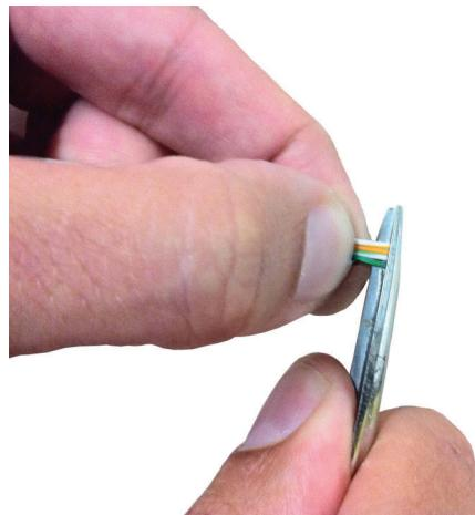
7. Insert the wires into the RJ45 connector, still holding them tightly between your fingers. The connector tab should be facing downwards and not visible. The insulating sheath should just reach the edge of the connector.
