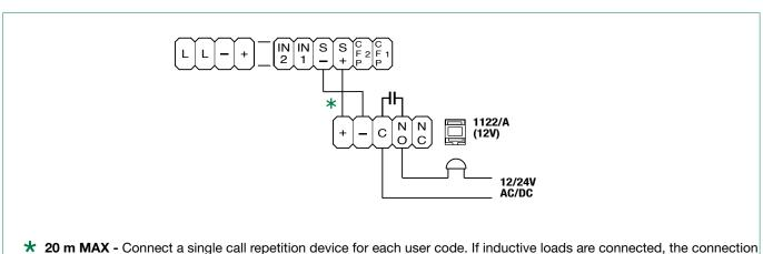
of 470nF capacitance in parallel with the C-NO contacts of Art. 1122/A is recommended
