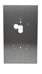
Plate allowing installation of the Extra, Ciao and Quadra external units in 1- and 2-module flushmounted boxes by Comelit, Bticino and Urmet. Dimensions (LxHxP): 137x236x2.5 mm.
