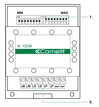
1. MIN and MAX microswitches define respectively the lowest and highest user codes which can be connected to the riser. (see <u>Addressing table</u>)
