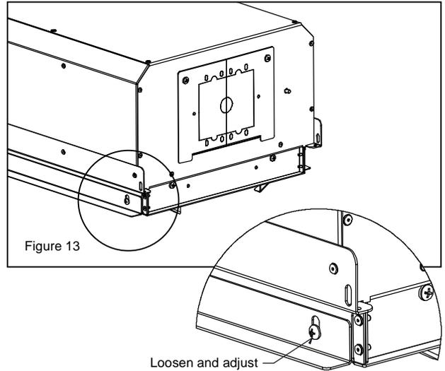
**NOTE:** Remove the cleat entirely to allow the enclosure to be mounted closer to the tile grid frame.
