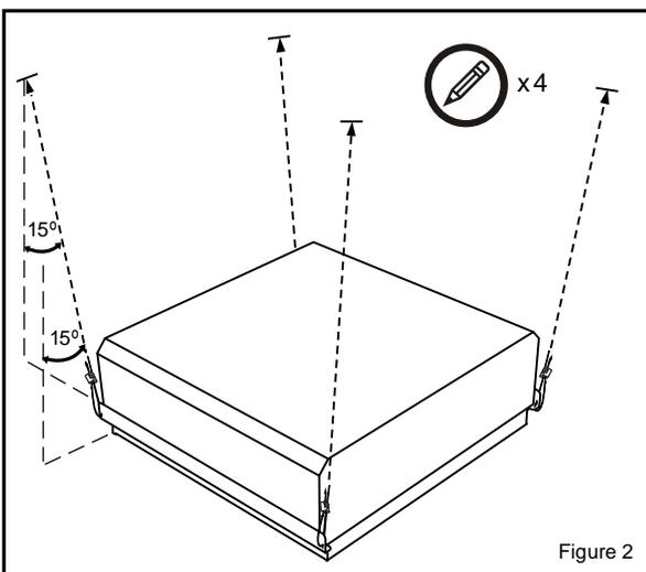
Examine ceiling structure (solid concrete, wood or steel truss) above kit to be installed to identify four support cable anchor locations. Each location should be approximately 15° outside of support holes in kit assembly. Mark locations with a pencil.
