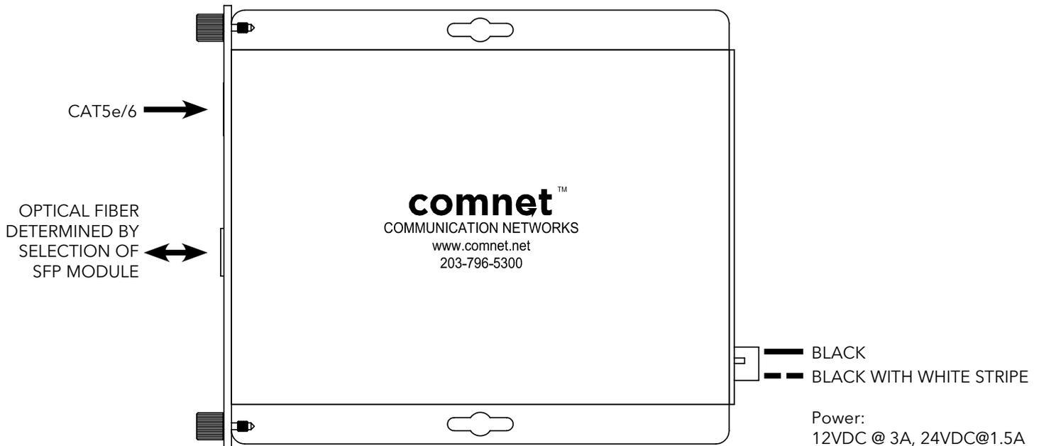
NOTE: Remove Electrical Connector for Rack Mount Units. **PoE is not supported when mounted within ComNet rack.**
