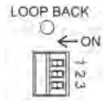
1. On one end (Head End), put unit into Loop Back Mode by setting Switch 3 to “OFF.” Switch 1 and 2 can be in any position. Data will not pass during Loop Back Test, LEDs may flash if data is sent during Loop Back Test.
