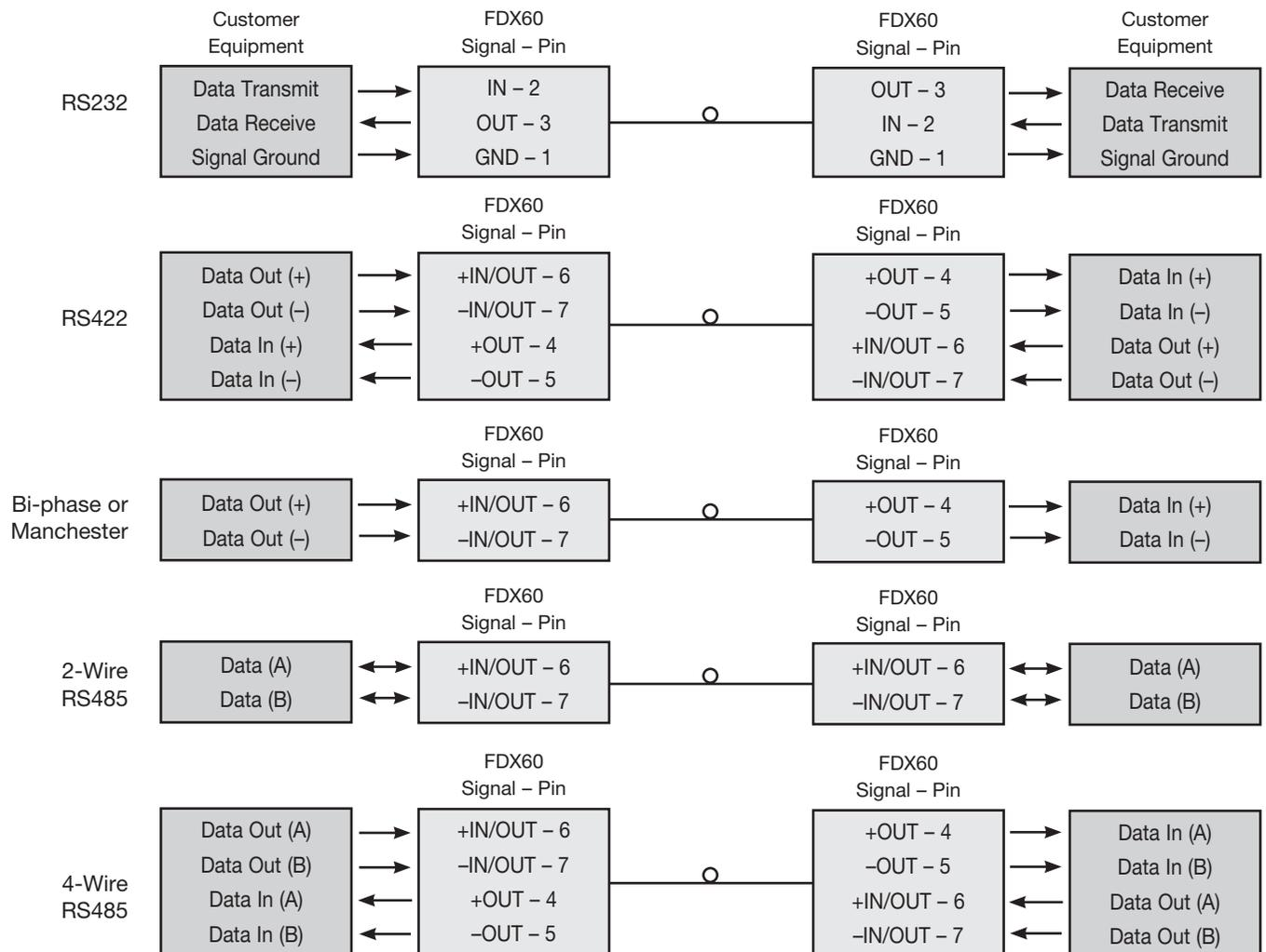
**FIGURE 13 – LOOP BACK TEST MODE**
