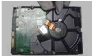
2. Screw the screws into the holes of HDD but not tighten them.
