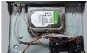
3. Put the HDDs onto the bottom of the device.
