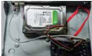
4. Connect the power and data cables.
