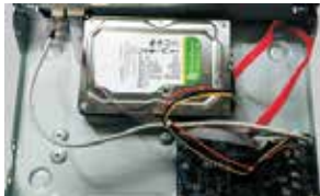
4. Connect the power and data cables.
