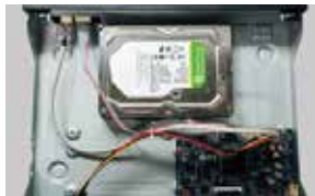
3. Put the HDD onto the bottom of the device.
