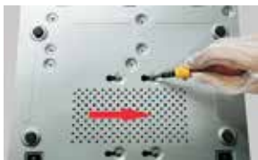
5. Turn over the machine and secure the HDD with the screws.
