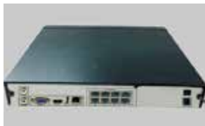
6. Install back the cover and secure it with the screws.
