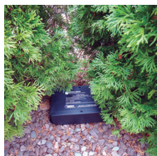
DA-610TO installation with the Sensor/Transmitter hidden under landscaping next to the driveway.
