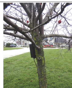
DA-611TO transmitter box 4 foot high in a tree for greater range Note: DO NOT mount a DA-610 on a tree.
