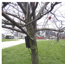
DA-611TO installation with the Sensor buried under the drive and the Transmitter hidden/mounted on a nearby tree.
