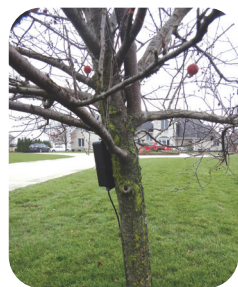
DA-611TO transmitter box 3-4 foot high in a tree for a range up to 1300 feet. Note: DO NOT mount a DA-610TO box on a tree.
