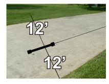
The ideal installation allows you to extend your detection range by installing the sensor under the center of drive.
