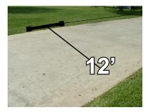
A typical installation is the probe 6 inches deep parallel to drive, which will allow the probe to "sense" 12 feet across the driveway.
