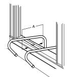
DIMENSION A: The windowsill width should be between a minimum of 6" (15 cm) and a maximum of 13" (33 cm).
