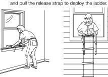
4. Exit carefully through the window and place your feet on the first rung. Hold onto the window frame until your weight is evenly distributed on the ladder. Climb down, keeping your body close to the ladder.
