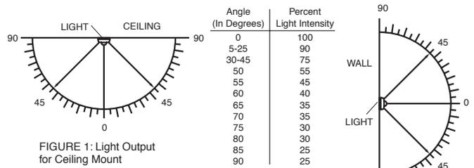
FIGURE 1: Light Output for Ceiling Mount
