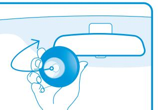
The suction cup is the Window Button front side (active part). This part should face the outside of the window.
