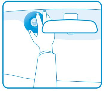
The suction cup is the Window Button Switch' front side (active part). This part should face the outside of the window.
