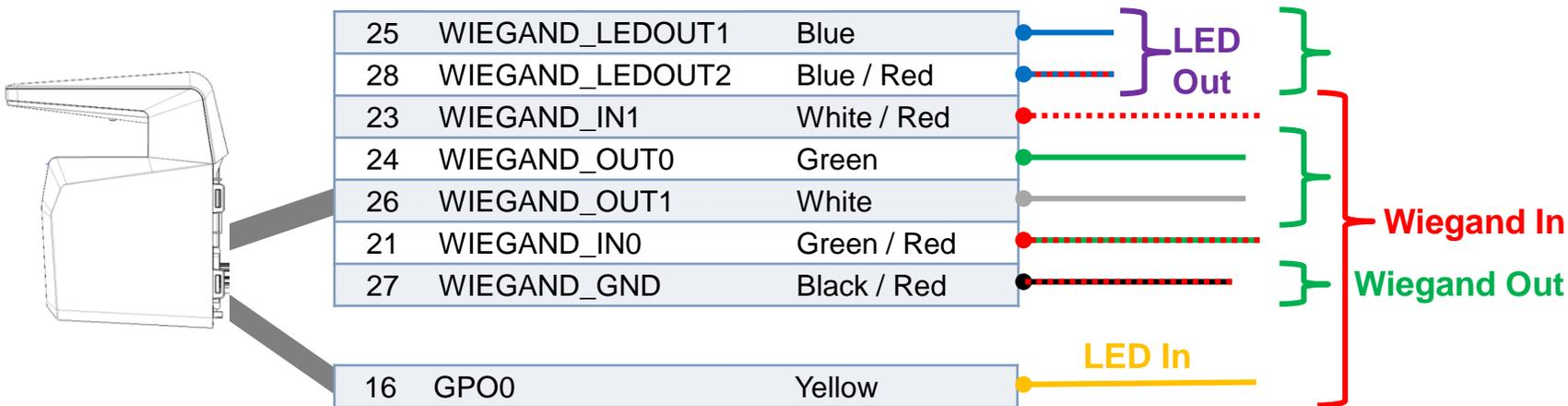
Three-conductor cable (shielded recommended) is required for Data 0, Data 1, and WGND.
