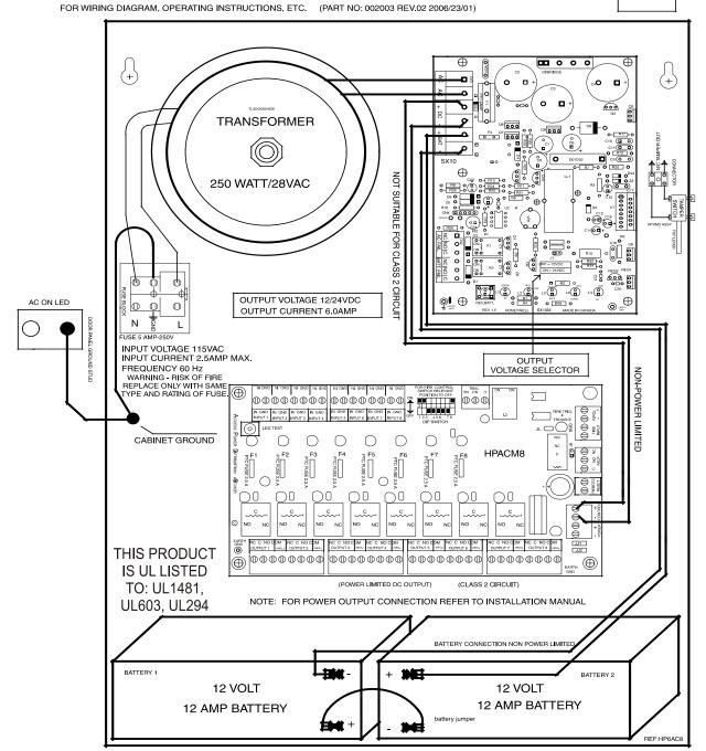
KEEP POWER LIMITED WIRING AT .25" MINIMUM SPACING FROM NON-POWER LIMITED
