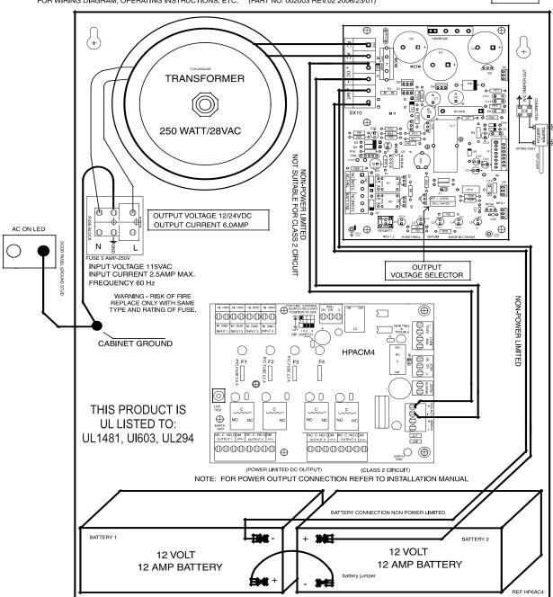
KEEP POWER LIMITED WIRING AT .25" MINIMUM SPACING FROM NON-POWER LIMITED
