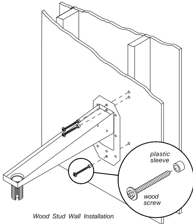
Wall Arms include three wood screws and plastic sleeves (left) for attachment to a wood stud wall. For attachment to a concrete wall additional fastener package **ACC 210** must be ordered.
