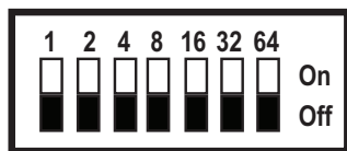
All dip switches are set to the default "OFF" position. (Device Not Addressed)
