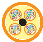
48-fibers (4 tubes of 12-fibers)
