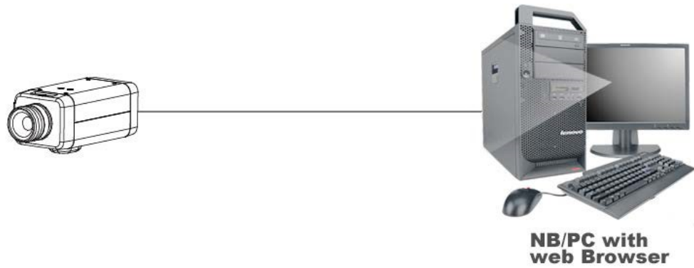
Figure 75 Illustra Flex Box Camera Network Topology Type II
