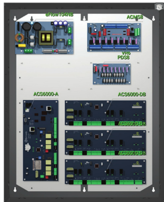
T2BV7F8S 8-Door Access System with Power
