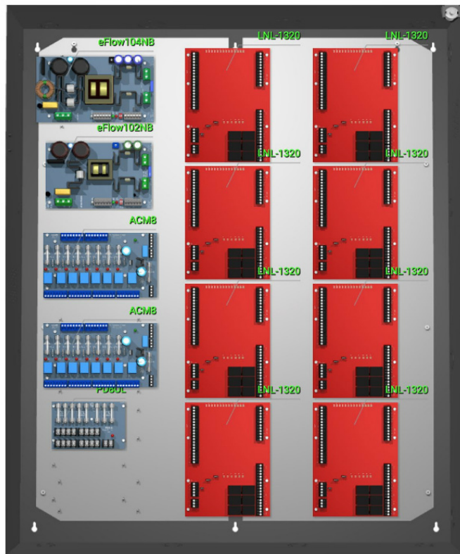
T3MK75F16 16-Door Access System with Power
