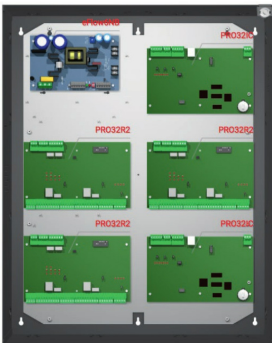
10-Door Access System with Power (ProWatch)
