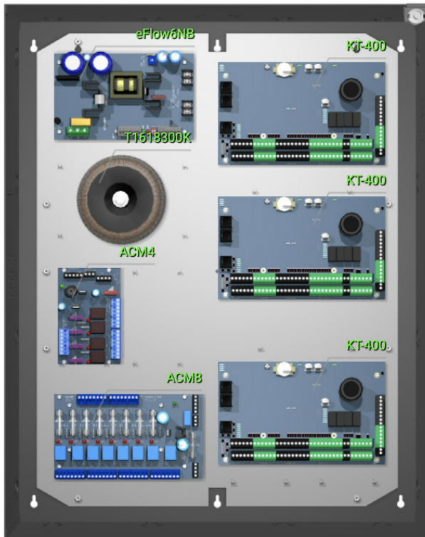
T2KHK3F12 12-Door Access System with Power
