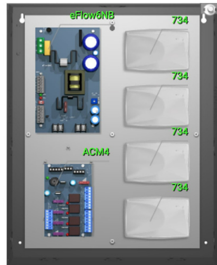
T1DMK3F4 4-Door Access System with Power
