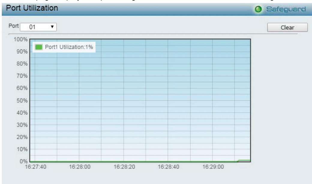
Figure 4.187 – Monitoring > Port Utilization
