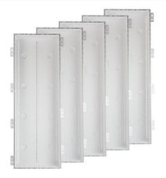
Constructed with a robust, wireless transparent ABS plastic material, this lightweight, low-profile enclosure is designed to integrate wireless devices into traditional structured wiring installations. The enclosure mounts easily for both surface and recessed applications., The hinged door and trim ring ENP4260-NA (ENP4260-5NA Bulk Pack) purchased separately to complete installation during trim-out phase.
