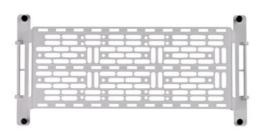
The On-Q mounting plate, AC1050, is constructed of WiFi transparent ABS plastic and is designed to securely mount a variety of 3rd party deives into the On-Q plastic structured wiring enclosures. The mounting plate can be mounted vertically or horizontally and include (4) plungers and grommets along with velcro strapping for devices to be safely secured inside the enclosure without compromising wireless performance.
