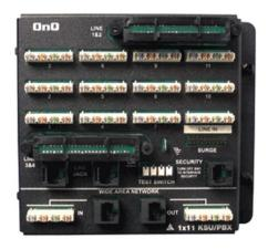
A module that can support up to 11 phone outlets for basic service, and can be upgraded for KSU/PBX service with the KSU Interface Kit (363490-01). Also supports a high-speed Cat 5e connection to one data outlet for broadband data services. 6"H x 6.5"W
