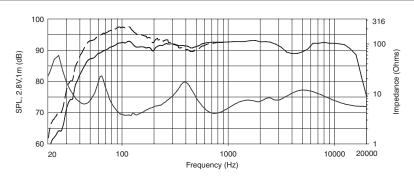
Frequency Response, on axis in half-space  $(2\pi, dotted)$ line) and full space ( $4\pi$ , solid line) at thru ( $4\Omega$ ) setting, Input Impedance.
