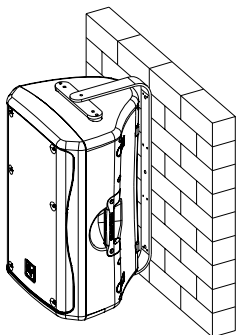
Kit Used - MB5 Wall/Ceiling Mounting Bracket (Wall Configuration)
