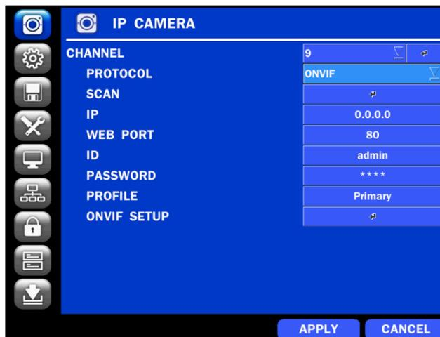
Figure 4.1.2 IP CAMERA Setup Screen (ONVIF)
