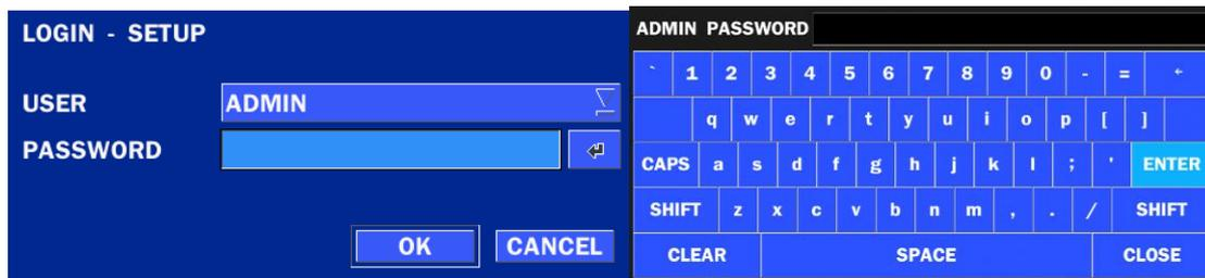
When the NS prompts the LOG-IN window, enter the PASSWORD using the virtual keyboard, or the front panel, or the remote control. For ADMIN, the factory default password is 1111. It is highly recommended to assign a new password to protect the system. User can assign a new password in SECURITY setup menu.
