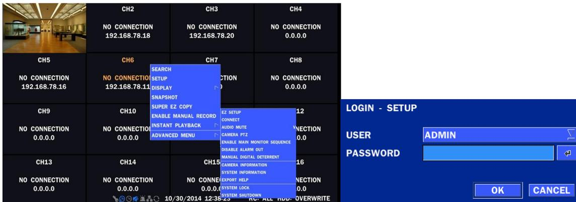
2. Go to SETUP > SYSTEM > DATE & TIME SETUP
