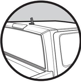
**Truck:** Cable routed into side door.
