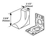
Eliminates need to offset 2400 Series Raceway when connecting with surface panel boxes. Has 3/4" and 1" concentric trade size KOs with 1" trade size KO elongated so adjustment from surface to center of bushing is 1" (25mm) minimum to 1 5/8" (41mm) maximum. Has twistouts for transition to 1500 and 2600 Series Pancake Raceways.
