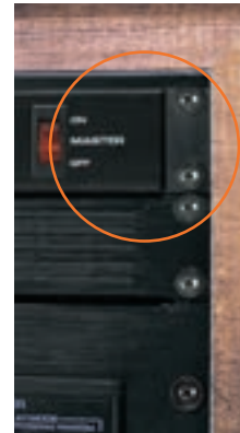
without trim strip installed
