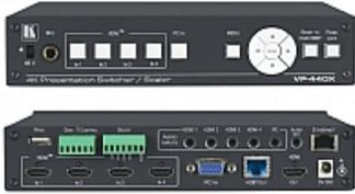
VP-440X is a high-performance 18G 4K HDR presentation switcher/scaler with four HDMI inputs and one computer graphics (VGA) input. It scales the video, embeds the audio, and outputs the signal to two identical outputs – one HDMI and one HDBaseT – together with an analog stereo audio output. Via HDBaseT, it extends video signals to up to 40m (130ft) over CAT copper cables at up to 4K@60Hz (4:2:0) 24bpp video resolution and provides even further reach for lower HD video resolutions
