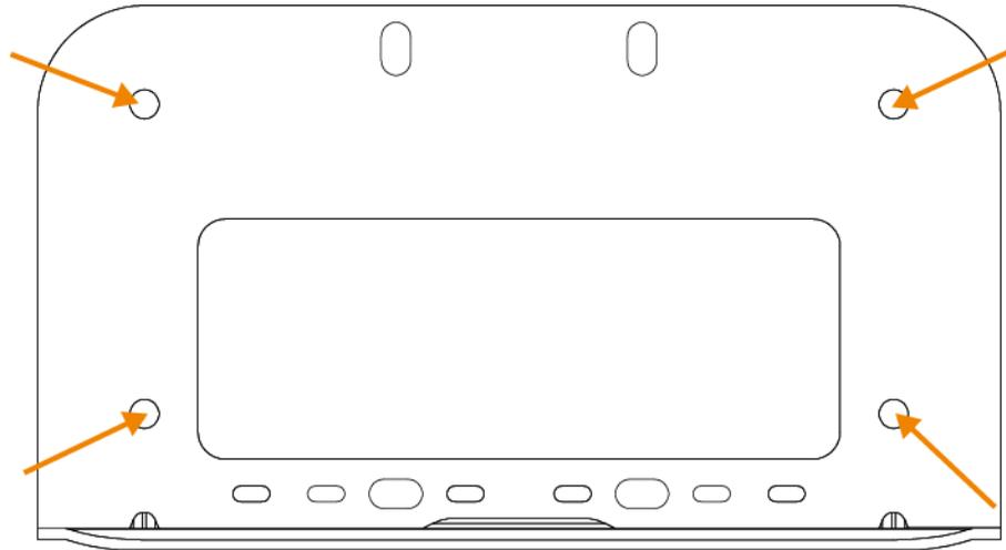
2. Secure the wall mount bracket on the wall within screws.
