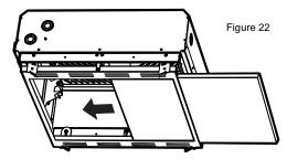
3 Push panel assembly back into place and rotate latches to lock position.
