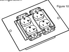
4 If outlet box configuration is attached to wiring/conduit prior to box attachment, remove two-piece electrical plate from box sidewall, feed configuration through large opening. Then re-attach two-piece plate to close around conduit.
