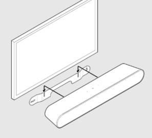
If your TV is wall-mounted, align the top edge of the bracket with the bottom of your TV, leaving at least 2.5 inches (mm) between them.
