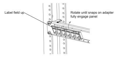
Note: Adapter housings can be installed with or without terminated connectors installed in them.
